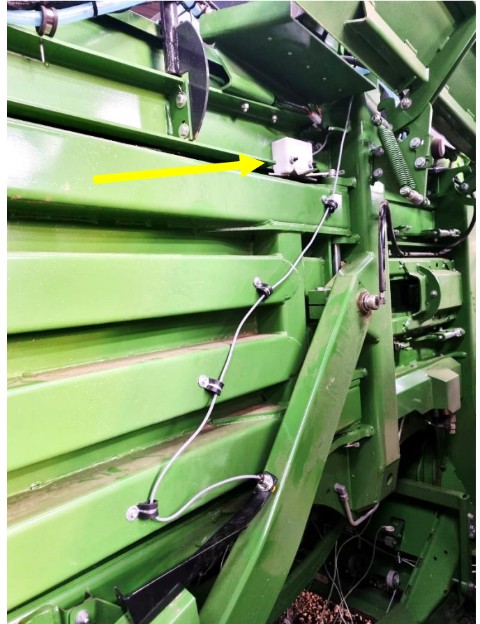
Star Wheel Mounting location shown for the LH side; Star Wheel mounting is same for the RH side.
