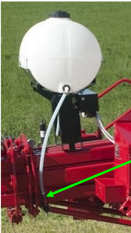
Example drain/Fill line on the baler
