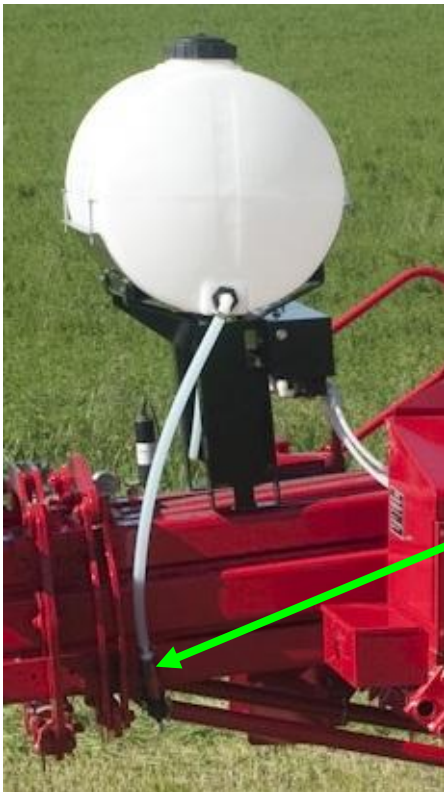
Example drain/Fill line on the baler
