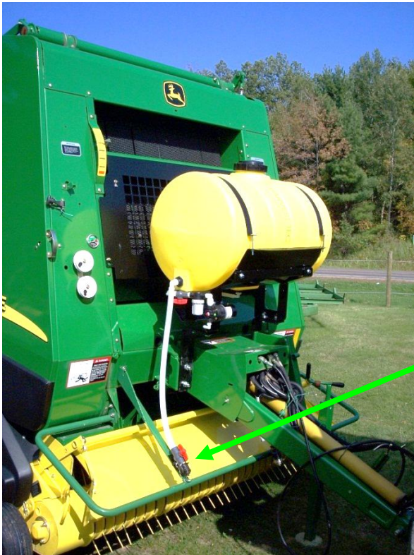
Example drain/Fill line on the baler
