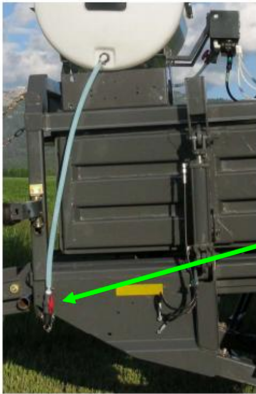
Drain/Fill line on the baler
